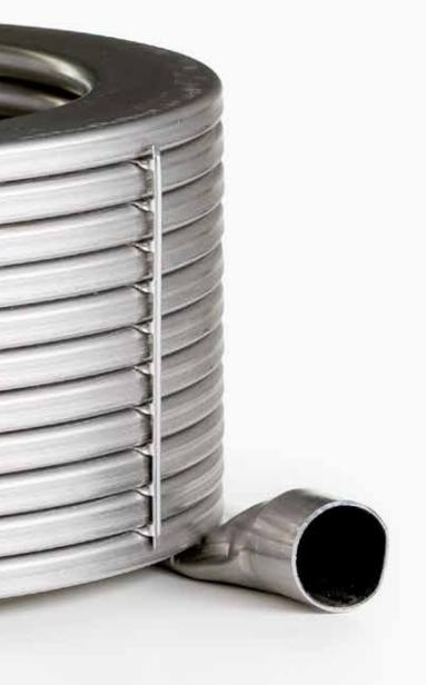
Italtherm has designed and developed a **new stainless steel heat exchanger** with extra wide water passages: the inner section of the coils has been increased by 4 times in comparison to the market standards.
